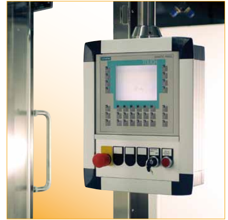
III.: Control via touch screen
