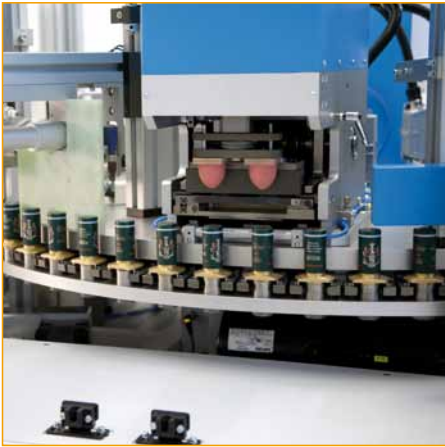
Combination example "Top Spin LC" (circular printing) + "Speed Modul" (top printing) printing of LongCaps (closures).
