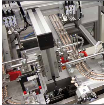
Partial view: printing parts feeding
