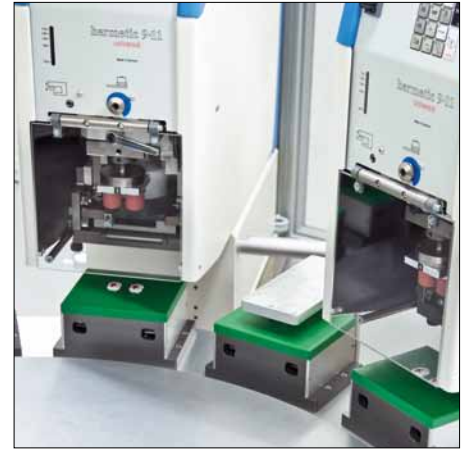
Intermediate drying station for printing "wet in wet"
