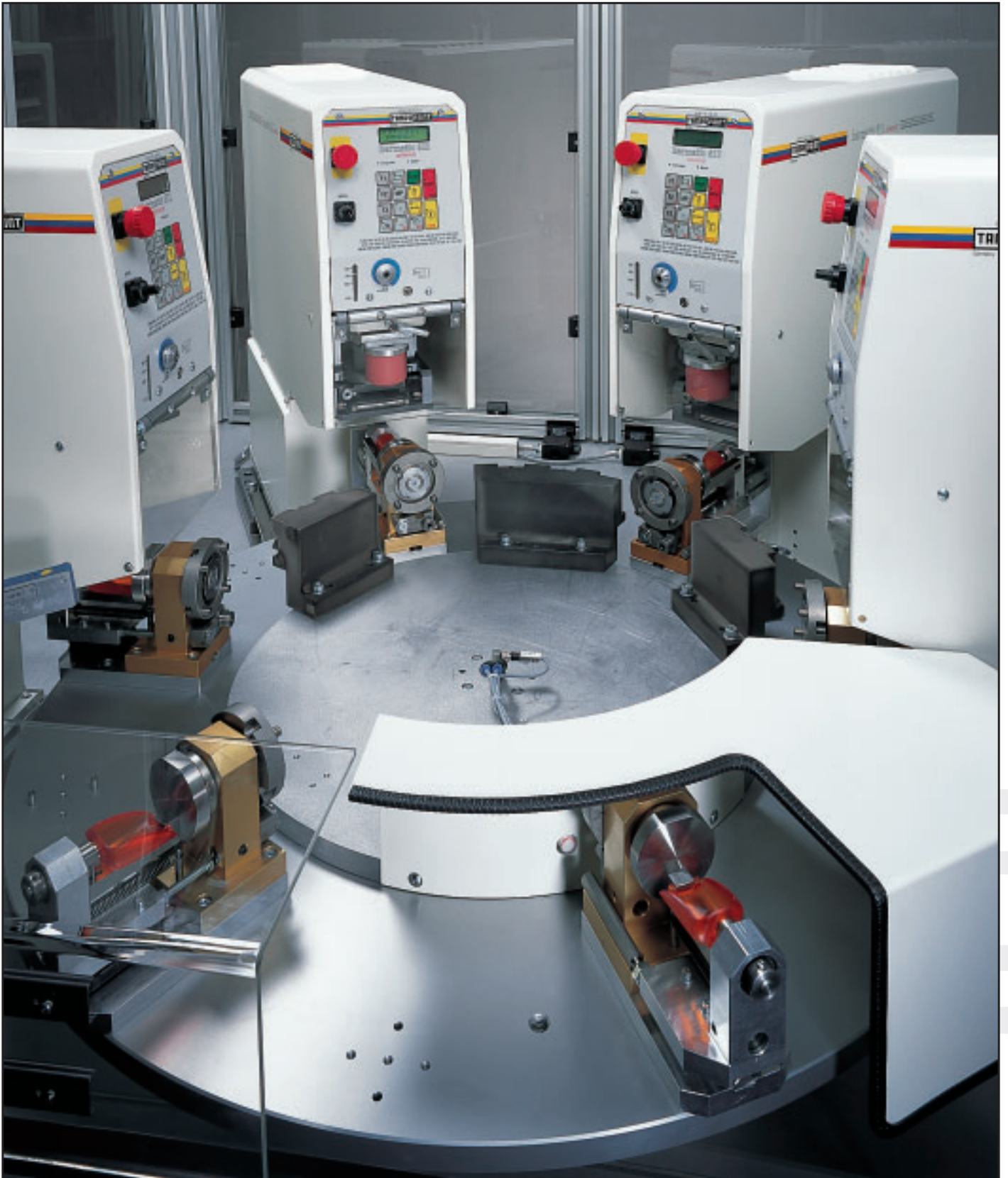
Modul 2000 with 4 Hermetic 6-11 and rotary jigs
