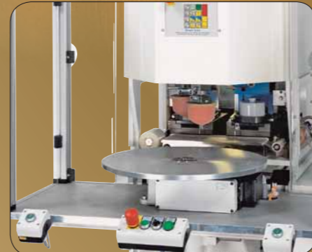
"T2" rotary index table for the feeding of workpieces
