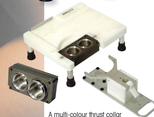
A multi-colour thrust collar can also realise 4-colour printing, i.e. 2 ink/docting cups per cliché unit.
